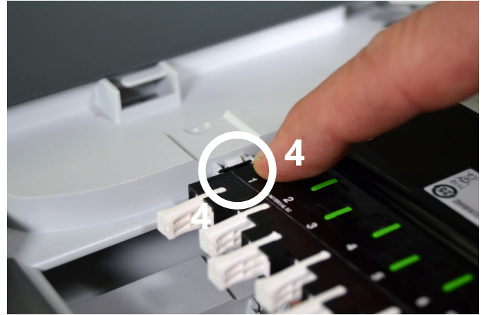
6.11. Push in snapping feature number 4.
