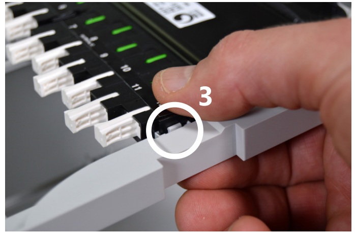
6.10. Push in snapping feature number 3.
