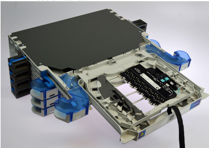
6.15. LC-MPO Module installed
