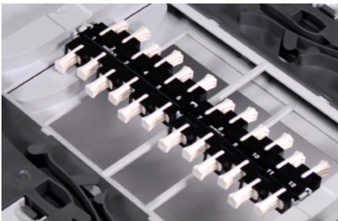
8.3. Align the Adapter Packs.
