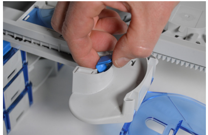
7.2. The retaining feature can be opened (hinged back) if additional space is needed (optional).
