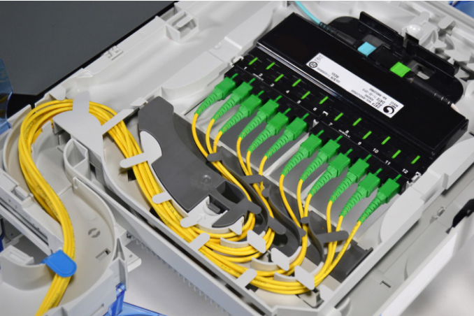
7.4. Route the patch cords through the first bend as illustrated. Use 3 patch cords per bend control for the SC-MPO Module. Clean the connectors before installing!
