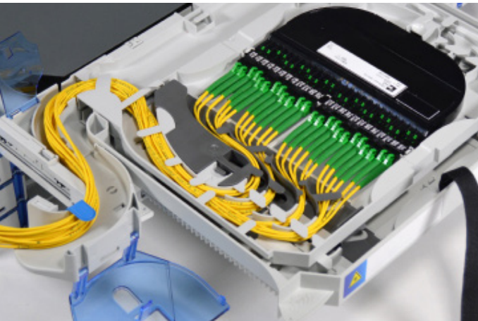
7.5. Route the patch cords through the first bend as illustrated. Use 6 patch cords per bend control for the VA Module. Clean the connectors before installing!
