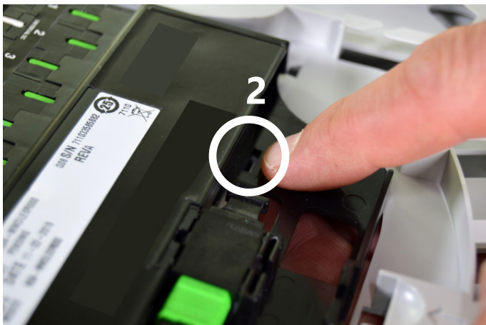
6.9. Push in snapping feature number 2.
